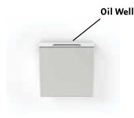
NOTE: Steamhead to be installed 6-12" above the finished floor. A 1.5" diameter hole in the steam room is required to mount the steamhead. Refer to the Mr.Steam Installation Manual for additional installation information.
